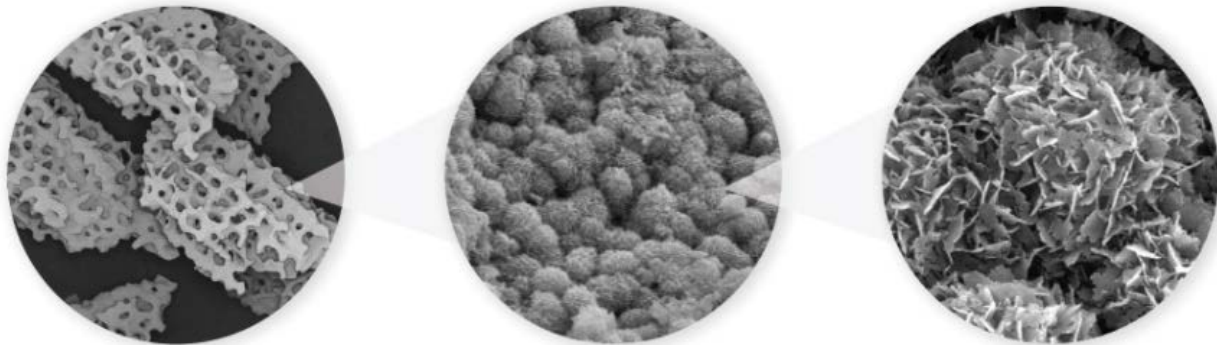
Biogenix TrelCor granules shown at 25X, 500X, and 20,000X magnification, respectively. Under high-powered scanning electron microscope (SEM) visualization, the nanocrystalline HCA surface is apparent.
